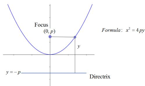
Note: You are used to using  $y = ax^2$  where  $a = \frac{1}{4p}$
